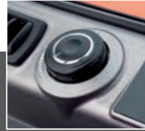
RPM dial / Auto idle Thanks to the electronic control, the optimal engine rpm can be set per workload. The auto idle function applied as standard helps fuel efficiency and reduces noise levels.
