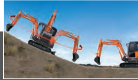
Higher gradeability and work capability Thanks to the high tractive effort and strong swing torque, the DX62R-3 & DX63-3 offer excellent capability for working on slopes.
