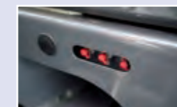
Centralised greasing points To make maintenance easier, the greasing points have been centralised.
