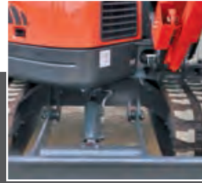
Boom swing The swing bracket and the boom swing cylinder size ensure powerful and stable performance.
