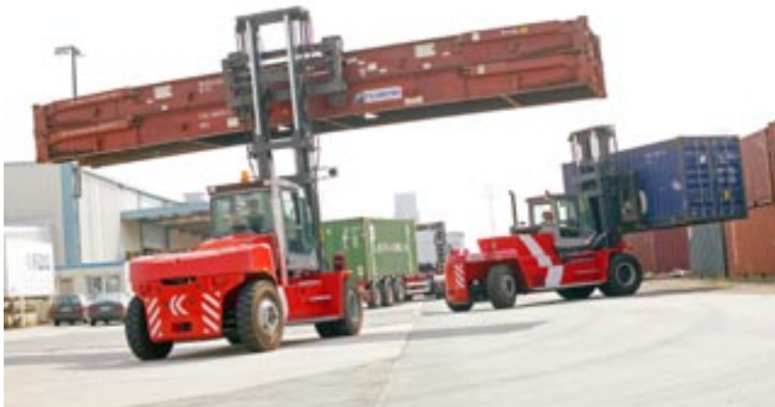
All masts from 3 to 8+1 high are designed according to the free visibility principle.
