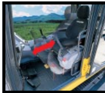
Seat Sliding Amount: 340 mm 13.4", increased 120 mm 4.7"
