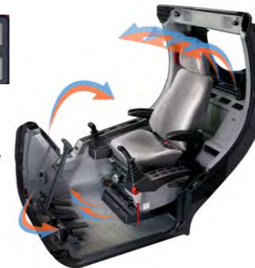
Visibility has been improved in all directions and the size of the cab has been increased.
