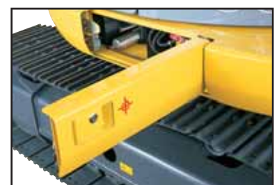
A large tool box provides plenty of space. Grease pump storage space is also provided.
